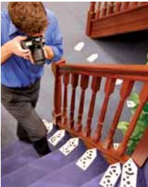
Most Minivator dealers use the Minivator eSurvey system for surveying curved staircases. This specially developed electronic system maximises the accuracy of a curved staircase survey whilst minimising the time needed to carry it out.
